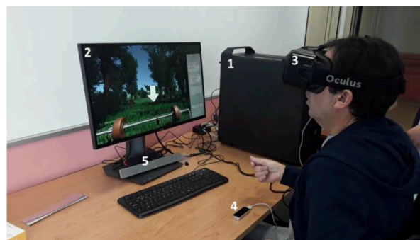
Figure 11. Virtual reality workstation used for poststroke rehabilitation with computer, monitor, speaker, Oculus Rift HMD, and Leap Motion Controller. From [15].
