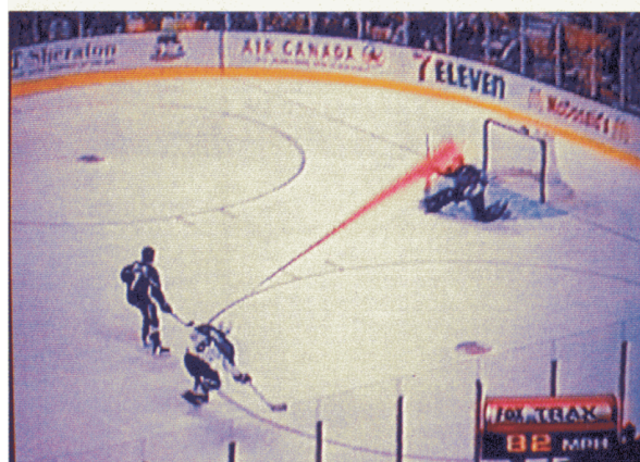
Figure 2. The FoxTrax system adds a glowing highlight in real-time to a moving hockey puck and “comet tail” to indicate the speed of a shot, also displayed in an inset (lower right). From [5].
