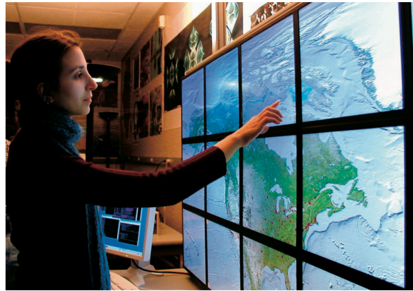
Figure 6. GeoWall 2 uses an array of LCD panels driven by PCs as a high-resolution interactive environment for large format geovisualization. From [9]. (© 2005, used with permission of the Electronic Visualization Lab, Univ. of Illinois Chicago and the GeoWall Consortium.)
